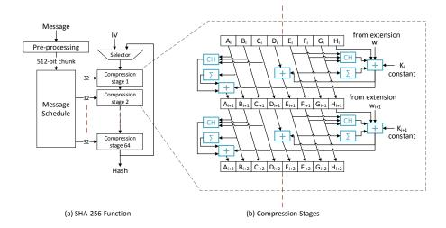
Figure 2: SHA-256 algorithm block diagram. (a) SHA-256 execution flow, including preprocessing stage, message schedule, which outputs 64x32-bit words, and 64 compression stages. (b) Detailed diagram of two 256-bit wide compression stages. Each includes 6x32 pass-through connections, two 32-bit adders, one 5-element and one 7-element. In addition, the compression stage includes permutations, selectors and majority functions.
