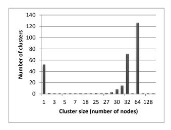
Figure 4: Histogram of cluster sizes in the Bitcoin SHA-256 accelerator. The biggest group includes clusters with 64 nodes, hence it matches the compression stages. The second biggest group includes clusters with 32 nodes, hence it matches the message schedule stages.
