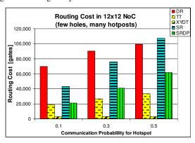
Figure 8. The routing costs as a function of hotspot traffic(few holes, many hotspots): 34X cost reduction by XYDT; 2X by SRDP
