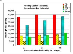
Figure 9. The routing costs as a function of hotspot traffic in typical NoC: 8X cost reduction by XYDT; 2.5X by SRDP
