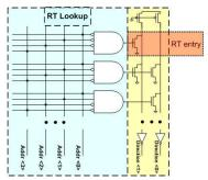
Figure 2. Efficient implementation of a static routing table
